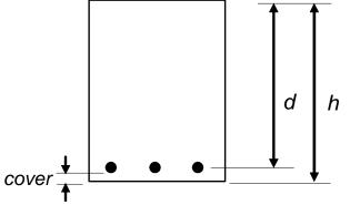
d - the effective depth of the section = distance from the top of the section to the centre of area of the reinforcement
