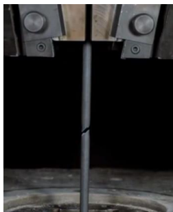
Tensile failure of a mild steel specimen
